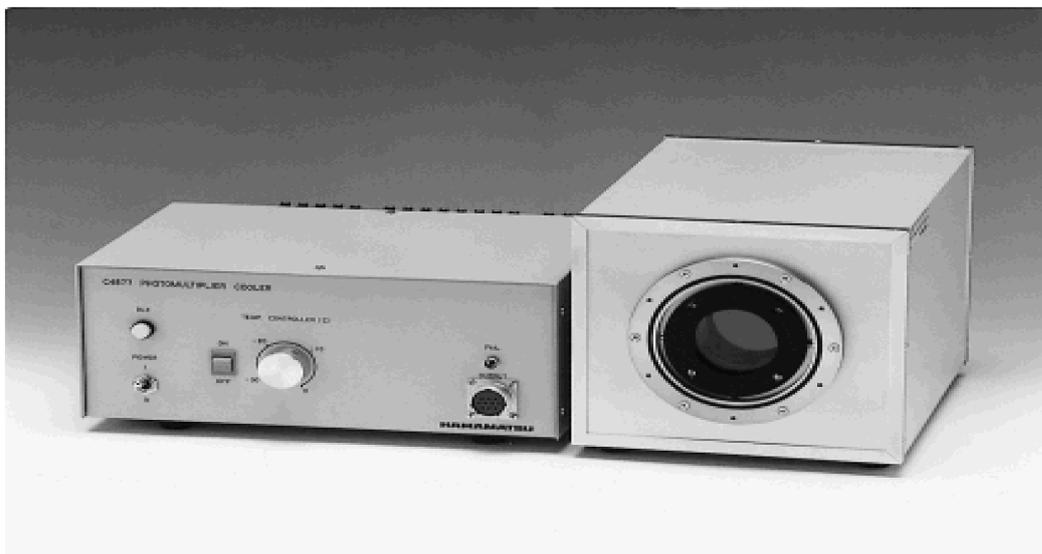
**Figure 2.13:** Hamamatsu C-4878 model PMT and power supply which are used for photon measurement(64).
